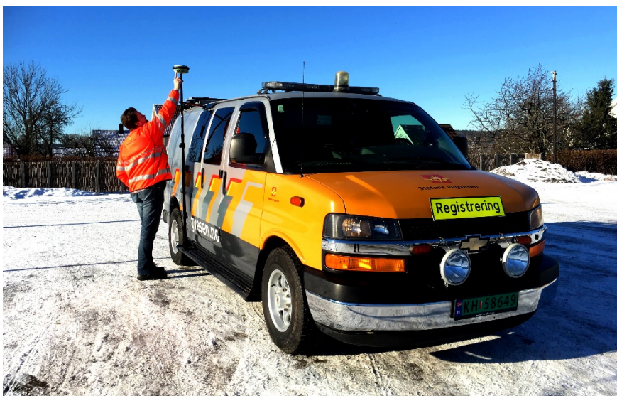
Figure 4-2: The road registration vehicle with the attached GNSS receiver
